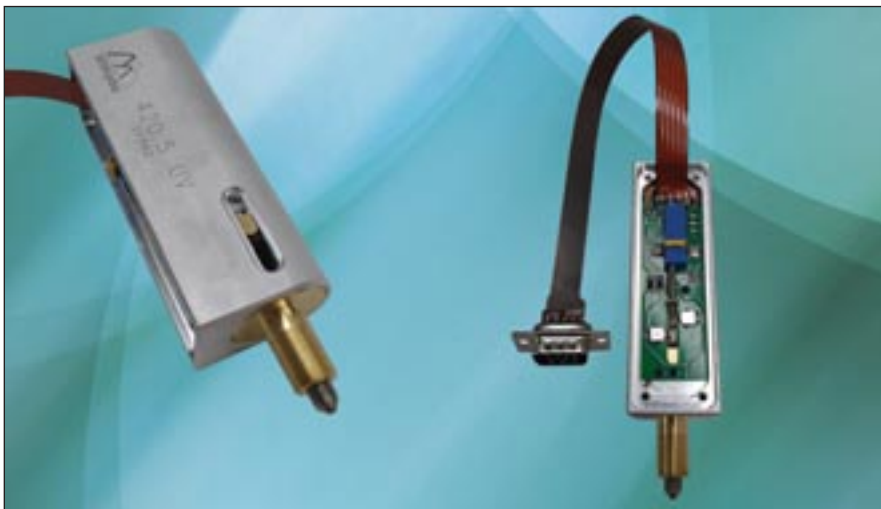
Figure 4. An economical solution to position feedback is provided by mounting a low-profile circuit board with a linear potentiometer, inside the Siskiyou actuator.
