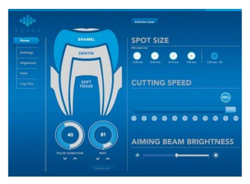
The convergent Dental laser system stores numerous scanning patterns that create cuts and holes like various traditional drill bits. These patterns are selected by the dentist from a point and click intuitive control software screen.
