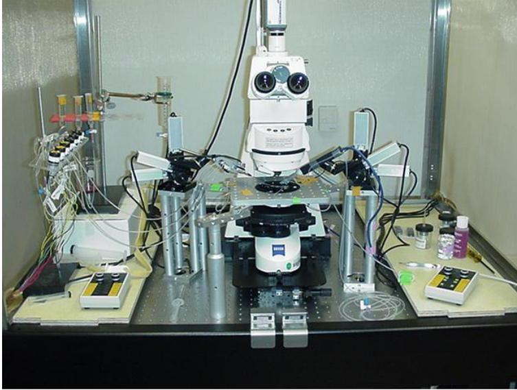
*Figure 3. In electrophysiology studies, the confined experimental space under a microscope objective means that the micropipette electrode(s) can only be introduced in a very narrow range of angles.*
